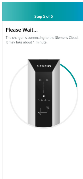
Step 5 – Wait for the charger to connect with the Siemens Cloud. For information about the LED lights during commissioning, see the Wi-Fi LED Light Sequence When Adding a Charger table under section 5.2 above.
